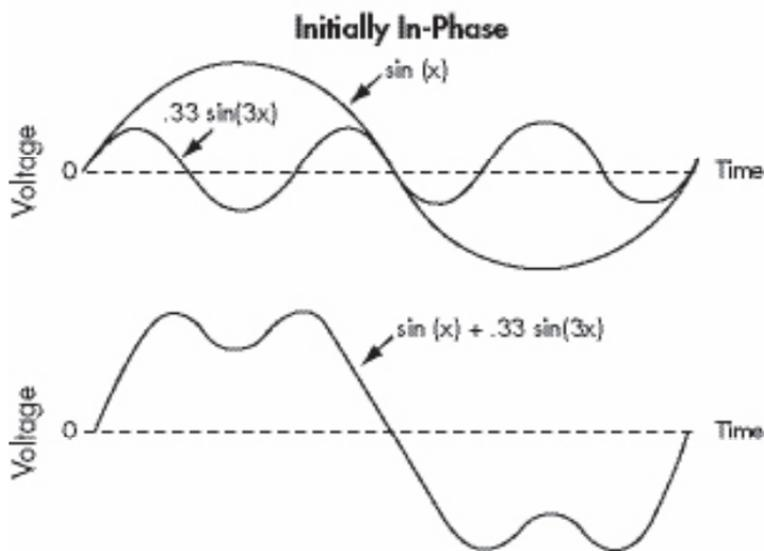
In this example, the two waveforms begin in-phase with each other, and produce a distorted waveform with a flattened top. The composite waveform can be changed by adding the same harmonic, initially out-of-phase with the fundamental, to obtain a peaked effect:
