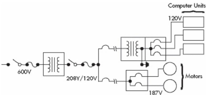
A transformer establishes a separately derived power source. The transformer can be of the step-down type to reduce the supply voltage to the utilization voltage of the equipment or an isolation transformer if the supply voltage is already at the appropriate voltage.
