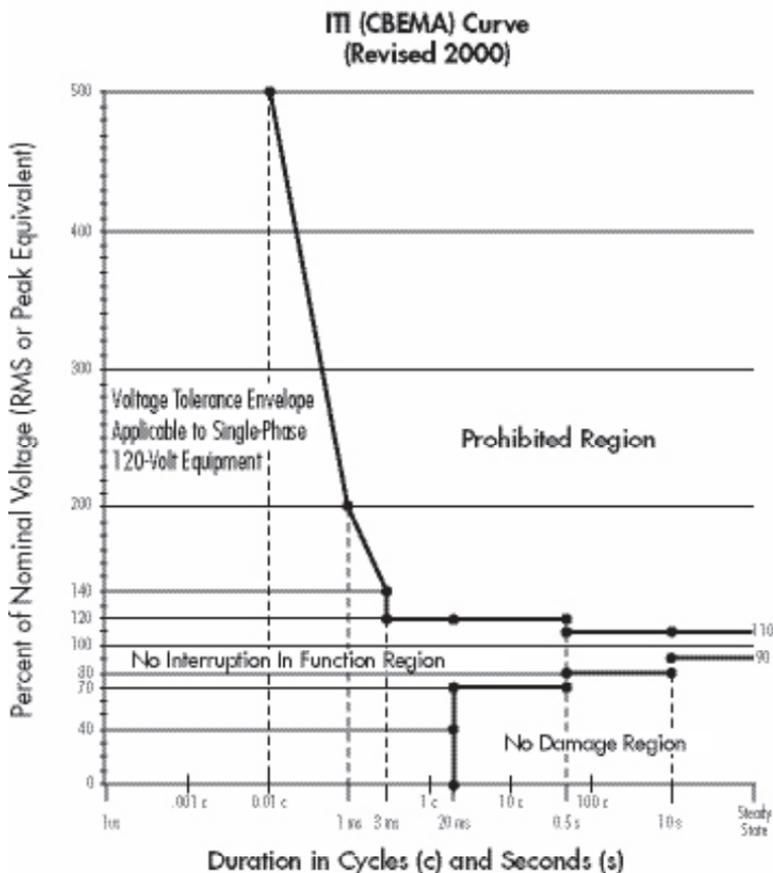
The susceptibility profile implies that computers can tolerate slow variations from -13% to + 5.8%, and greater amplitude disturbances can be tolerated as their durations become shorter. In fact, many computers can run indefinitely at 80%
