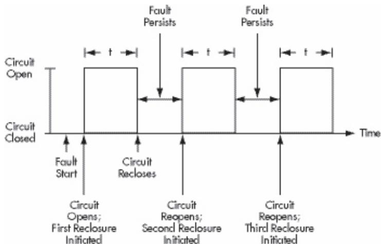
Normally a few seconds are required to clear a fault and energize the appropriate circuitry for a reclosure. The reclosing interval for a recloser is the open circuit time between an automatic opening and the succeeding automatic reclosure. In the above diagram, three intervals of duration 't' are
