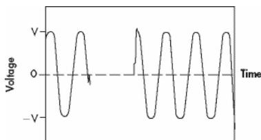
Total loss of input voltage. Often referred to as a "blackout" or "failure" for events of a few cycles or more, or "dropout" or "glitch" for failures of shorter duration.
