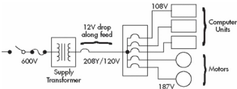
If the feeder has a resistance of 0.075 ohms, during a motor start the voltage drop along the feeder is:
