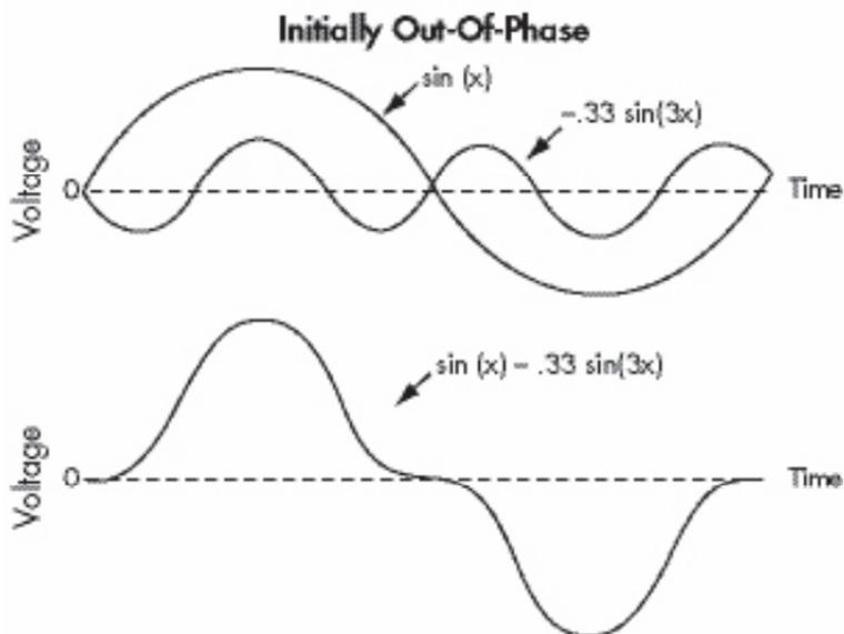
Harmonics can be differentiated from transients on the basis that transients are not periodic and are not steady state phenomena.
