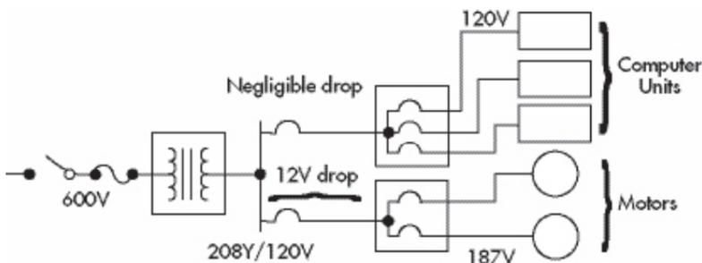
An even better approach is to effectively create a new supply system for the sensitive loads by using a transformer in addition to a separate feeder
