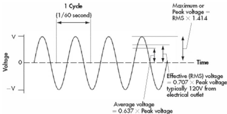
Any variation to the voltage waveform, in magnitude or in frequency, is called a power line deviation. However, not all power line deviations result in disturbances that can cause problems with the operation of electrical equipment.
