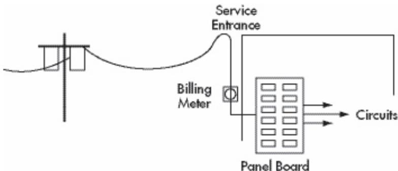
In larger distribution systems this power panel board will supply other panel boards which, in turn, supply circuits.
